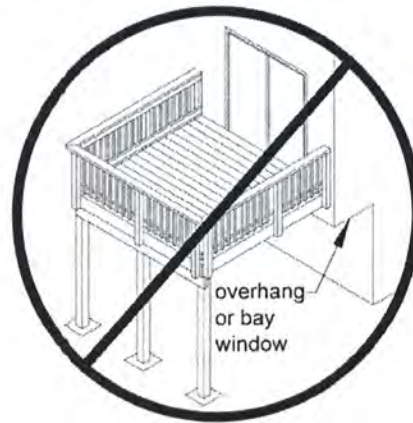
Figure 18: No Attachment to House Overhang
